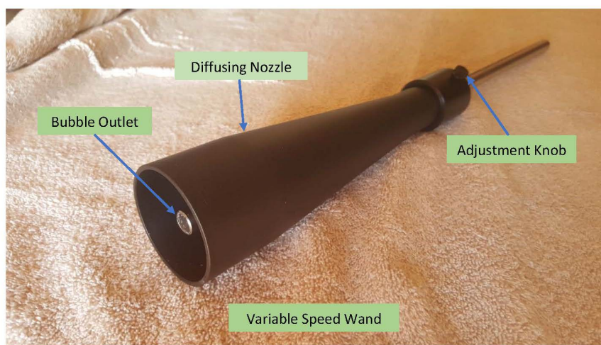
Figure 8 — Variable-Speed Wand: Adjustment Knob, Diffusing Nozzle, and Bubble Outlet.
